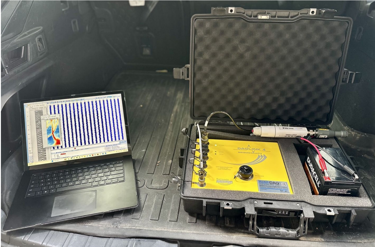
Figure 3. The ReMiDAQ™ Bundle in action at a job site for an Earth Tech IBC / ASCE Site Class project at Minden, NV, USA. The ReMiDAQ™4-12 or 24 channel seismograph includes wireless connection to your field laptop and everything you need to determine the depth and thickness of subsurface layers, IBC site class, and produce a report in the field, in about 30 minutes (Figure 1).
